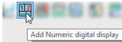
The digital display panel opens and a new digital meter is added to it, yet without a signal assigned. The easiest way to transfer a signal to the digital display is to drag and drop the signal out of the signal tree.
