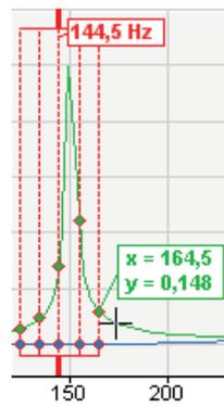
Harmonic component and sideband markers can be displayed in combination, too. The figure below shows a view with a harmonic marker below and two above the main marker. The sideband offset is set to 10 Hz.
