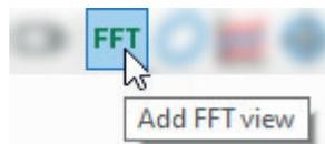
You can move individual or several highlighted signals from the signal tree to the main view of the FFT view using drag & drop. In the case of an InSpectra module, you can drag the entire module into the FFT view. In doing so, relevant parameters for the FFT view are copied from the module settings.
