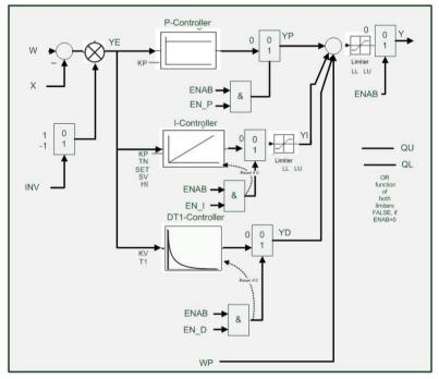
Figure 51: Block diagram of a universal PIDT1 controller
