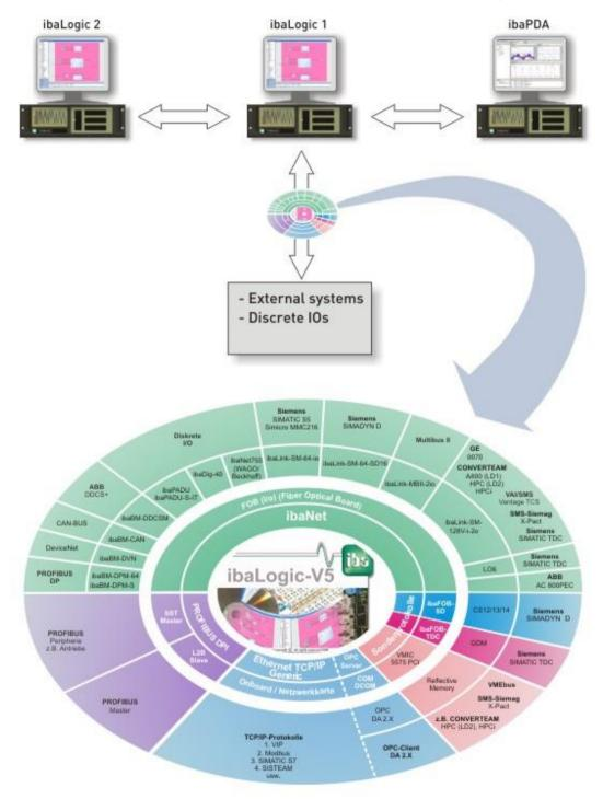
Figure 6: Connectivity to iba and external systems
