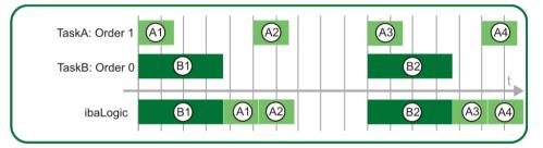
Figure 143: Task evaluation with time shift
