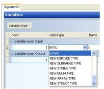
Figure 80: Creating a data type in a function block
