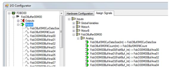
Figure 118: Assigning input signals
