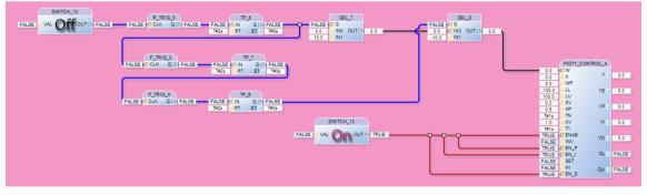
Figure 59: PIDT1 controller with signal trends
