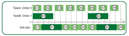
Figure 146: Task evaluation with time shift (reversed priority)
