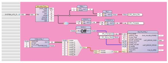
Figure 44: Example: CONCAT functions
