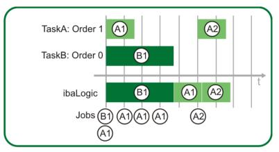
Figure 144: Task evaluation with time shift - Excerpt
