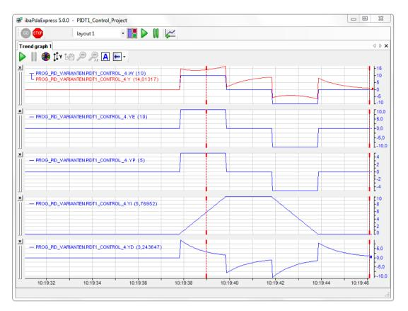
Figure 60: PIDT1 controller with signal trends
