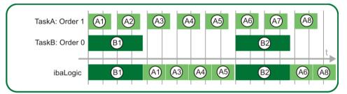
Figure 145: Task evaluation with time shift
