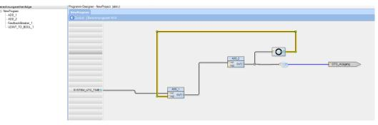
Figure 28: FeedbackBreaker as feedback point
