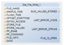
Figure 38: DAT\_FILE\_WRITE block
