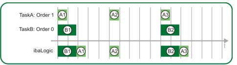
Figure 142: Evaluation without overflow – 2 tasks having different interval times, equal priority and a different order
