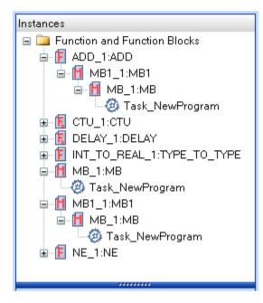
Figure 20: Instance view as a tree structure
