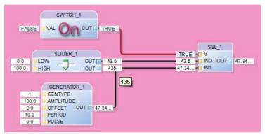
Figure 166: Generator output connected to the SEL output (OUT)
