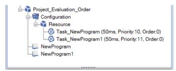
Figure 23: 2 tasks with identical interval time but different priority
