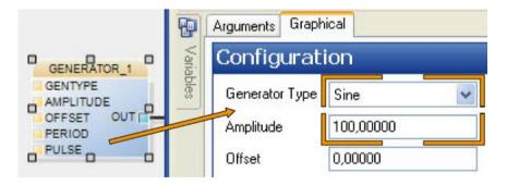
With this setting, the generator produces a sinusoidal waveform having a value between +100.0 and -100.0.
