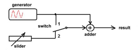
Figure 164: Circuit diagram of the sample exercise
