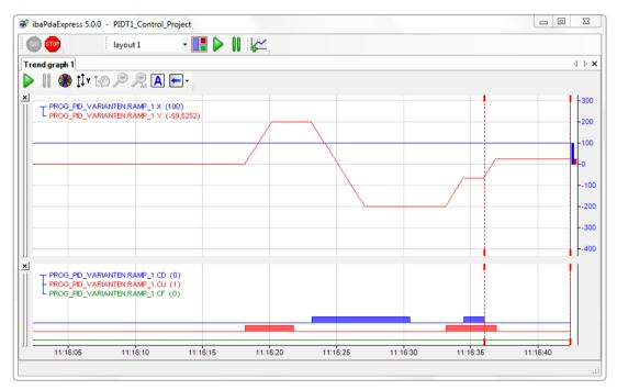
Figure 63: Controlling ramps
