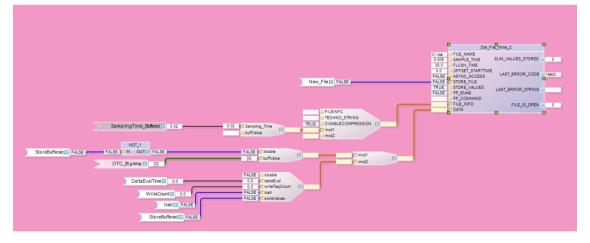
The DFW is operated with a sampling\_time of 5 ms. This corresponds to the event clock pulse. Module "mod2" is configured as unbuffered values.
