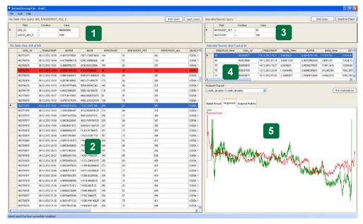
Graphical user interface of ibaDatawyzer-ICC: customized queries (1), matches result table (2), extended query (3), list of potential parent coils (4) and graphs for matches and alignments (5)
