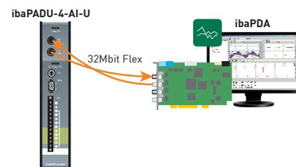
With ibaPADU-4-AI-U, the sampling rate can be up to 100 kHz in a point-to-point connection.
