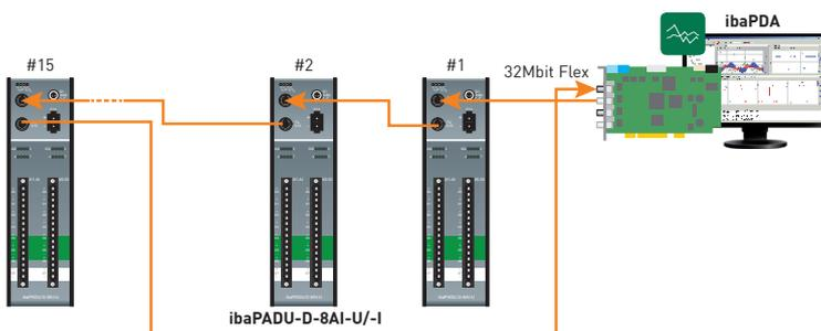
Up to 15 „32Mbit Flex“ devices can be connected to a „Flex“ ring.
