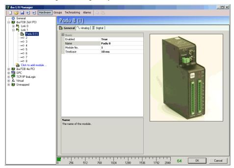
Click on the tab *General* in this dialog box and you can make the general settings for the module, such as module name, module number and sample time (if different from basic sample time).
