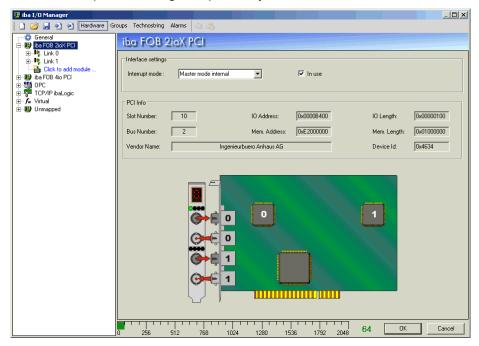
A mimic of the card is displayed in the dialog box when you mark the main branch of the card in the tree view.
