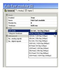
By selection of the link mode, i. e. data types, the signal tables of analog signals will be adjusted automatically. (Integer: Min / Max; Real: Gain / Offset)
