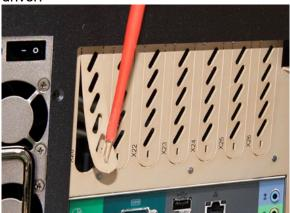
**3.** Above the slot, there is a screw in an opening, which is used to fix the card later. Loosen the screw and remove it.
