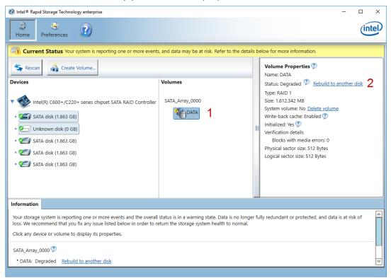
In the following dialog select the hard disk that you want to use to restore the redundancy of the RAID array.
