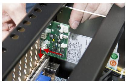
5. Fasten the card with the previously loosened screw.
