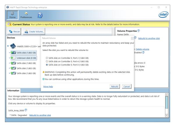
Click on "Rebuild" to start the process. The duration of the process varies depending on the hard disk capacity.
