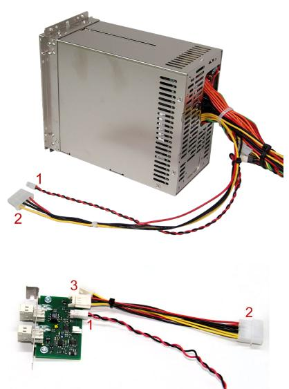
(1): Connection of redundant power supply unit: If a redundant power supply unit is to be monitored, connect the twisted cable (black/red) of the power supply unit (1 - picture above) to the 2-pin connector (1 - picture below) of the card. This connection is not necessary, when a standard power supply unit is used.
