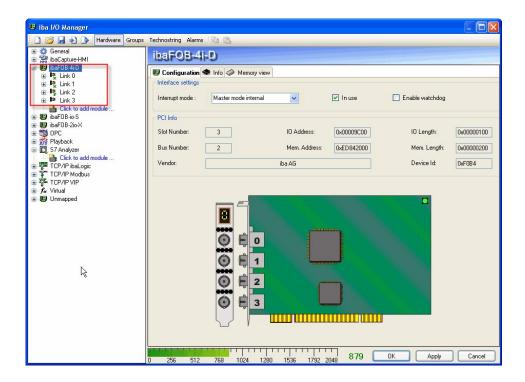
4 links are available in this example to connect the device (module). If the device should use the SIMOLINK interrupt, use at least the first link (Link 0).
