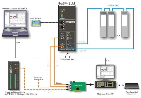
Figure 2: ibaBM-SLM with ibaPDA-V6
