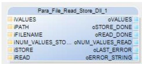
Figure 77: Para\_File\_Read\_Store\_DLL as a function block in the program
