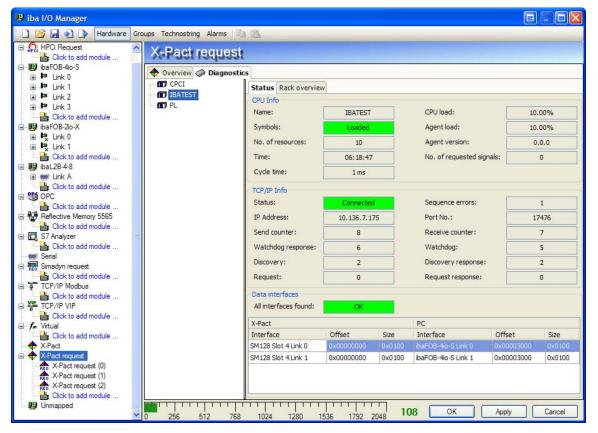
Connected CPUs send the rack configuration in their status messages. This rack configuration is shown on the Rack overview tab.
