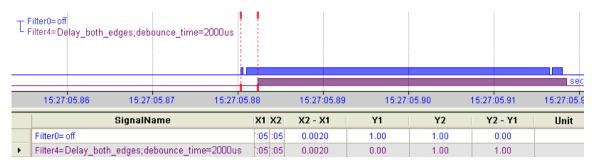
Figure 10: Debounce filter: "Delay both edges"
