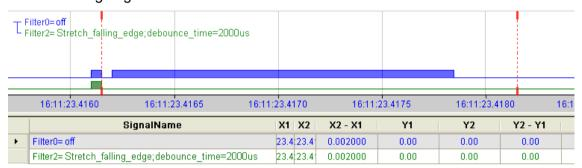
Figure 8: Debounce filter: "Stretch falling edge"
