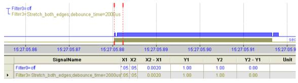
Figure 9: Debounce filter: "Stretch both edges"
