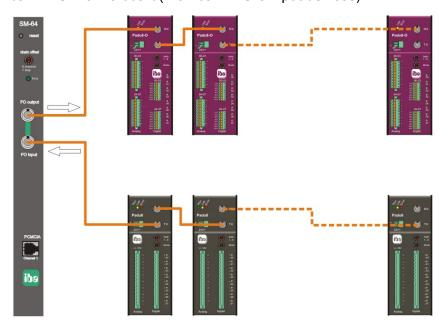
Figure 5: Daisy-chain with ibaPADU-8-O to ibaLink-SM-64-io
