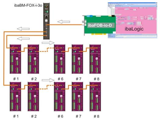
Figure 6: Process IO redundancy
