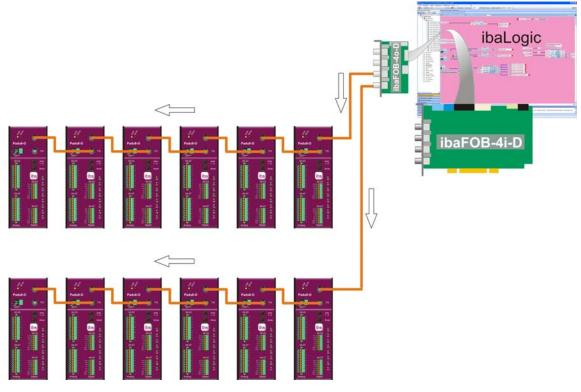
Figure 4: Multiple daisy-chains with ibaPADU-8-O
