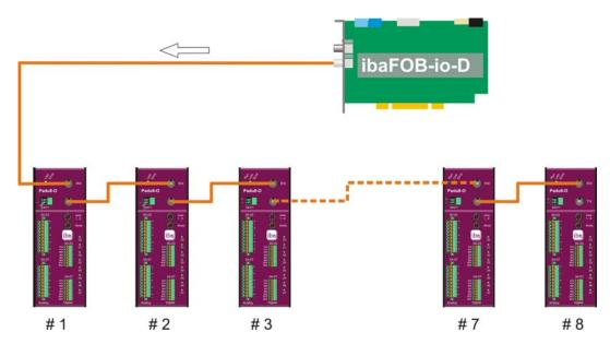
Figure 3: Single daisy-chain with ibaPADU-8-O
