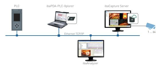
With ibaPDA-PLC-Xplorer and ibaCapture process data and video images can be recorded time-synchronously and be analyzed together in ibaAnalyzer.
