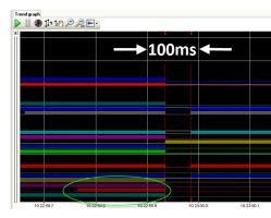
High speed ibaPDA fault capture trend of the S7 PLC's digital I/O's
