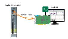
With ibaPADU-4-Al-U, the sampling rate can be up to 100 kHz in a point-to-point connection.
