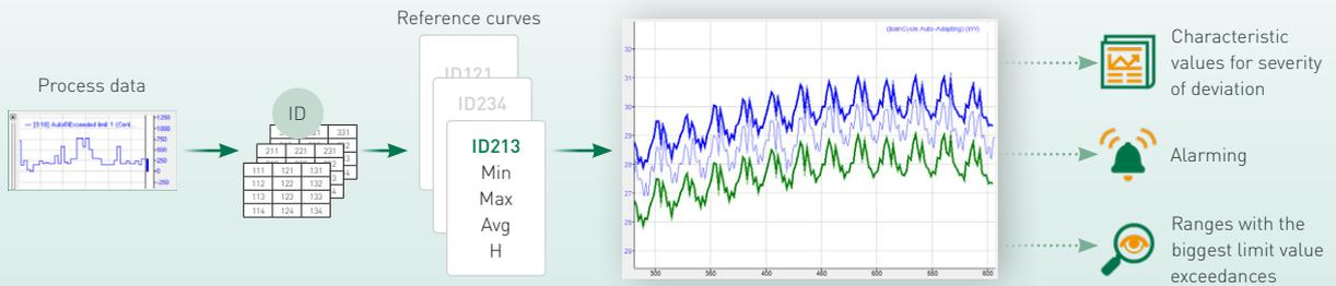
After the "good" curves have been learned for different process conditions, deviations are immediately displayed during the process.
