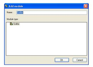
Enter a name and confirm with <OK>. The sniffer sub module is then displayed below the ibaBM-CAN module.
