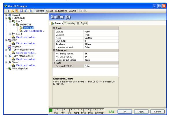
Figure 13: Sniffer module - General tab
