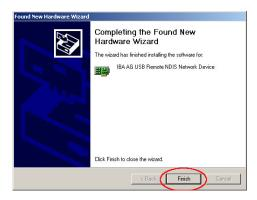
Now, the USB interface is available as an additional Ethernet interface to the device. You should now configure the interface in order to establish a communication to the device over the USB cable. Therefore, choose "Settings" in the Windows Start menu and then "Control Panel". There open "Network Connections" to see a list of available network connections.
