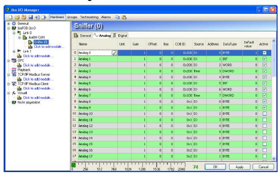
Figure 14: Sniffer module - Analog tab
