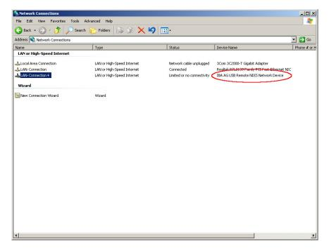
6. There, in section "LAN or High-Speed Internet" you'll find a LAN connection with the device name "IBA AG USB Remote NDIS Network Device". Highlight this line and select "Properties" from the "File" menu. A new dialog box "LAN-connection... Properties" will open.
