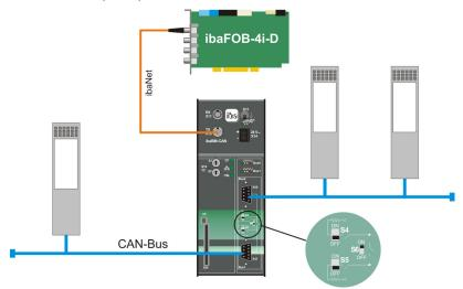
Figure 6: ibaBM-CAN in looping through mode
