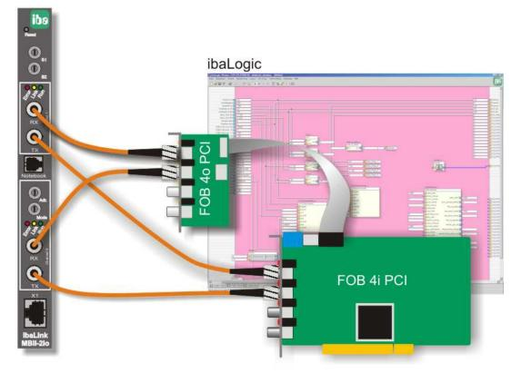
Figure 5 ibaLink-MBII with ibaLogic
