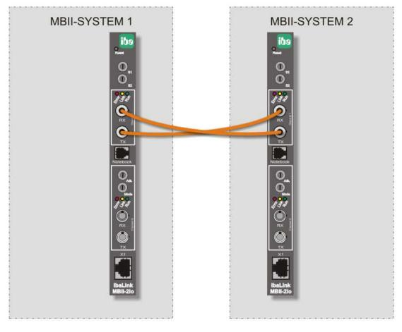
Figure 3 Peer-to-Peer operation (frame-to-frame connection)
