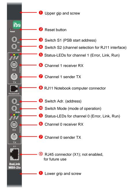
Figure 1 View on front panel of ibaLink-MBII-io
