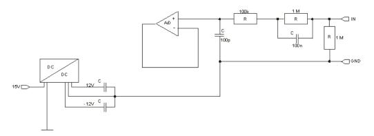
Figure 8: Simplified input circuitry of the ±10V input with ibaPADU-HI resistor network
