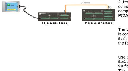
2 devices in a line structure connected to a notebook computer via ibaCom-PCMCIA-F card.
