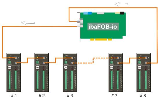
Figure 11: Ring topology for external synchronization of ibaPADU-8 devices
