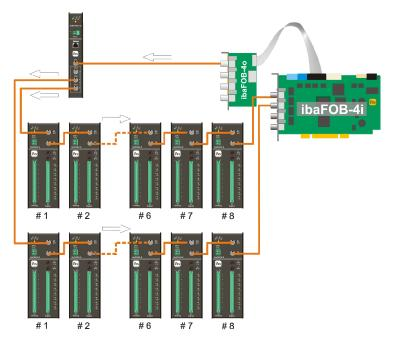
The first output of ibaFOB generates the clock for the FO-chains (e. g. 3.3 ms).
