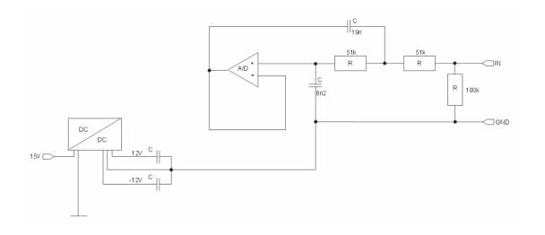
Figure 9: Simplified input circuitry of ibaPADU-8-F1 (250 Hz, 12 dB)
