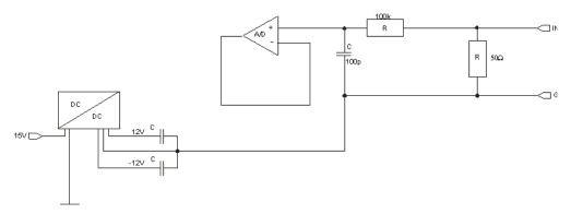
Figure 10: Simplified input circuitry of ibaPADU-8-I (±20 mA)
