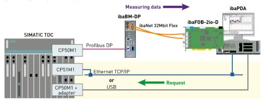
ibaPDA uses the interface of the Siemens programming device (PG-interface) for request handshake and the transmission of address books. Depending on the hardware and software installed, different access points are available for data acquisition:
