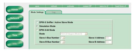
**5.** A click on <restart DP> reboots the device and simulation mode is active then.
