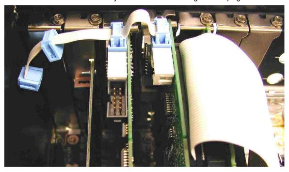
Figure 25: Connecting multiple iba cards by sync cable
