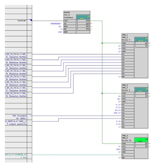
Figure 5: Configuration transmission channel with CTV\_P
