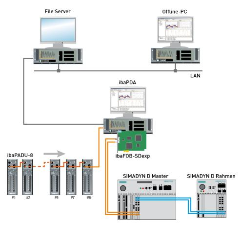
Figure 1: Example of configuration with ibaPDA
