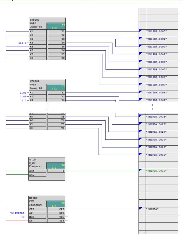
Figure 4: Configuration transmission channel with CTV
