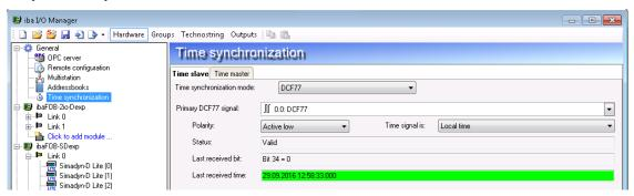
Figure 14: Time synchronization with DCF77-signal
