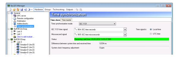
Figure 16: Time synchronization with IEC 1131 time signal
